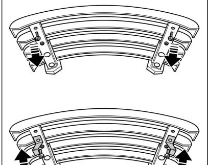
Figure 38. Fitting the hanging brackets to the firefront.
