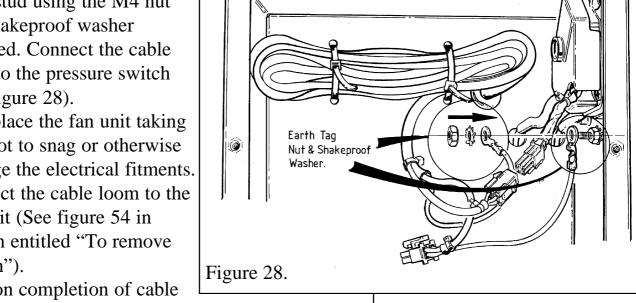
**8.** Upon completion of cable installation ensure that the loom and cables do not touch the horizontal surface of the fan casing immediately above the rectangular flue gas outlet. If cables run close or are in contact with this surface they should be held clear using the additional cable ties provided.
