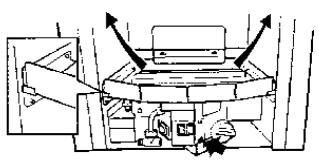
Figure 43. Burner unit removal
