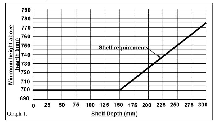
**3.1.9** The front face of the wall should be reasonably flat over the area that will be covered by the fire box top and side flanges to ensure a good seal. The minimum height from the top surface of the hearth to the underside of any shelf made from wood or other combustible materials is as follows:-
