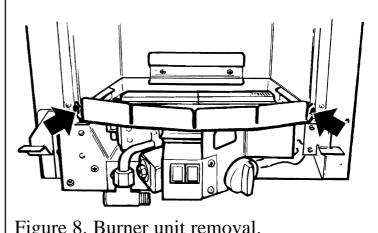
Figure 8. Burner unit removal.
