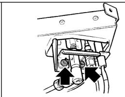
Figure 44. Pilot unit fixings (Dust cage not shown for clarity)
