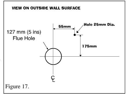
inside face. Add 18mm to this measurement to obtain the correct length of flue unit required. This measurement is for surface mounted flue box assemblies. Care should be taken if the flue box is to be recessed. *The fan box is not intended to be recessed into a timber framed building*.
